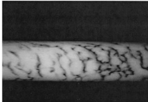
FIGURE 12. ‘Tiger’ waves for U = 1.0 \text{ m s}^{-1} (a) and U = 1.5 \text{ m s}^{-1} (b) in a 1" (25 mm) diameter pipe. They are like the waves that develop in core-annular flows and can be seen where the free milky water layer is thin. The released water is a dispersion of small clay particles water.
